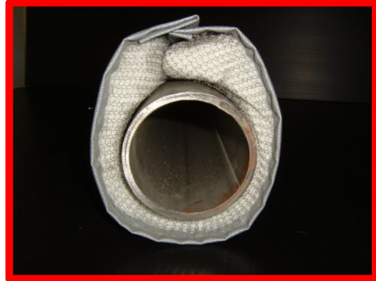
Needled insulation (fiberglass or silica) between outer layer of silicone or aluminized fabric and inner layer of stainless steel mesh.
